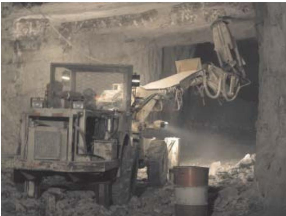
***“Scaling the back.” Removing loose rock from a tunnel (drift) at the Polaris mine.***
